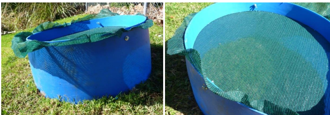
Figure 1. Cage design used for surface run-off and nematode field trials.
