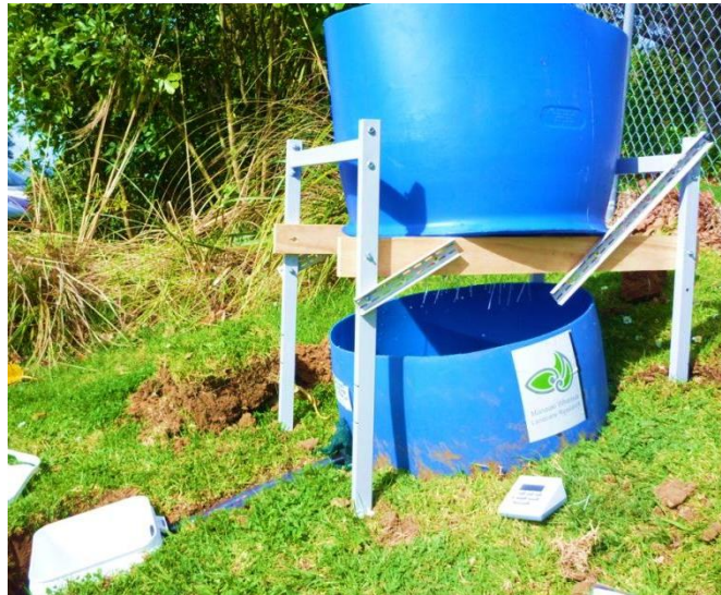
Figure 2. Rainfall simulator and cage (lid removed) setup for surface run-off experiments (in pre-trial testing before cages were set up in pasture).
